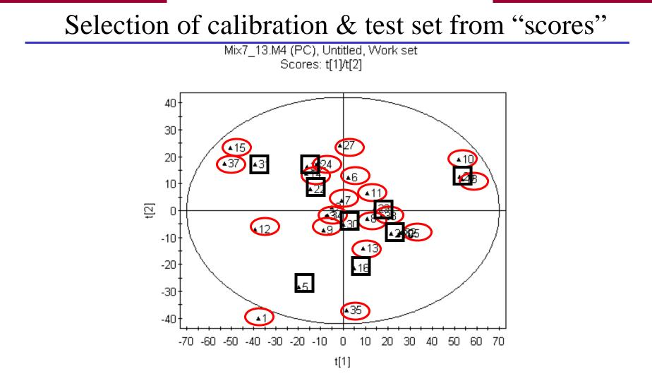
Calibration samples (circled) span the experimental space and are evenly distributed Over the whole surface.
