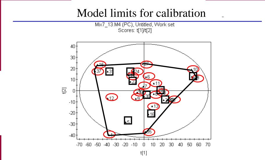
The black lines in the score plot define the limits for the calibration model. Within these limits the model will be valid.
