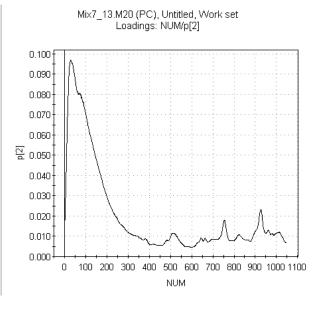
Loading (p1/wavelength) shows that the separation in the first PC depends on almost all wavelengths in the spectra. Loading (p2/wavelength) shows that the separation in the second PC depends on early wavelengths in the spectra.
